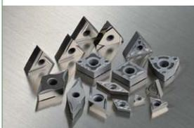
An uncoated cermet with a composite hard phase, which improves toughness and adhesion resistance. Ideal for continuous finishing of steel, cast iron, and sintered alloys at high speeds of  $v_c=300$ m or higher.
