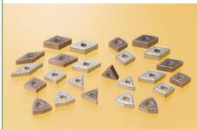
A chipbreaker series for exotic alloys and stainless steel, applications in which chip control is difficult. The EG Type is for roughing and general-purpose use and has spherical projections on its rake face to maintain chip control performance and thereby achieve excellent wear resistance and chip control. The EF Type is for finishing and has a rake angle focused on cutting performance (20°) to reduce wear and chip curl diameters and improve chip breaking performance.
