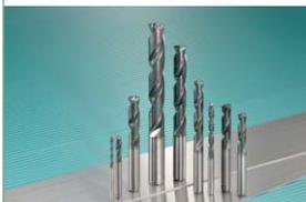
Enables high-efficiency drilling of cast iron at speeds of over  $v_f=1,000$ mm/min by applying RX THINNING, which drastically reduces cutting resistance, and a special double margin design to the cutting edge.
